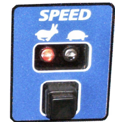
Regular or slow speed modes. Note: Machine is calibrated to always finish last pass on slow speed.
