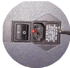
Main power switch Power cord input Main fuse box.
